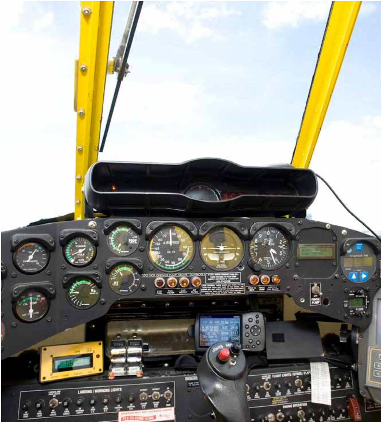
A satellite navigation system is mounted on the far right of this private spray plane's control panel. June 30, 2010. USDA Photo. https://flic.kr/p/8zybzv
